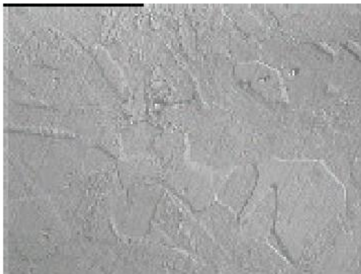
Figure6.34: Enlarged view of Microstructure of the surface away from CO 2 laser cut surface of stainless steel -304
