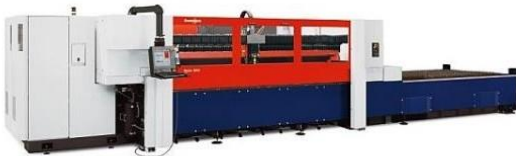
Figure 5.5 Bystar 3015 CO 2 laser cutting machine photograph
