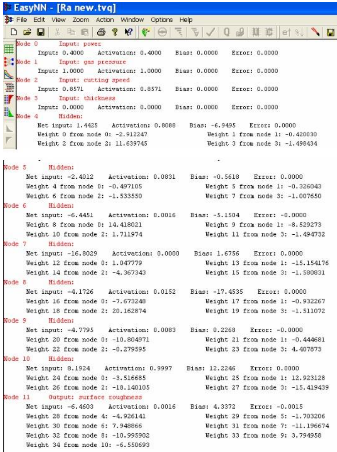
Figure 7.16: Weights of Multilayer Neural network Model with 4-7-1 architecture to optimise surface roughness in cutting stainless steel by CO 2 laser.
