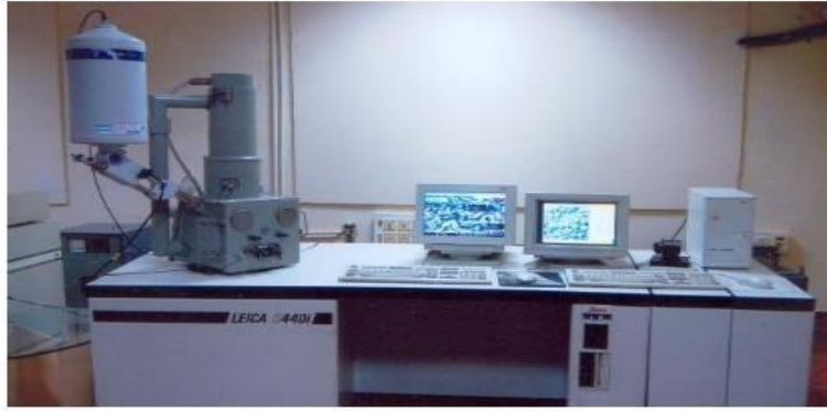
Figure 5.9 SEM image shows a Scanning Electron Microscope equipped with an Energy Dispersive Spectrometer and an Image Analyzer
