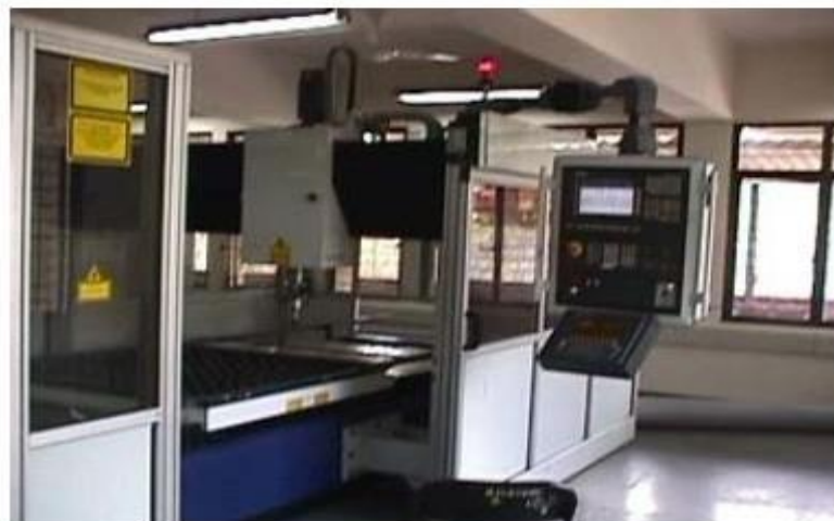
Figure 5.3 Laser cutting machine Rofin Sinar CO 2 (full view)
